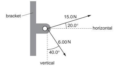
What are the magnitudes of the horizontal and vertical components of the resultant of the two forces?
