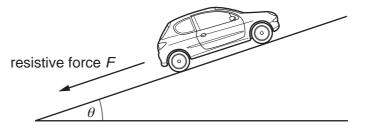
What is the force needed to propel the car at this constant speed?
